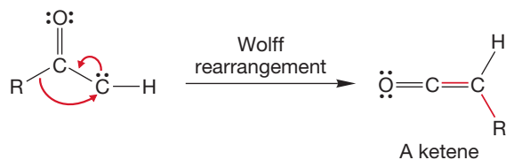
FIGURE 18.66 Intramolecular ketene formation from a ketocarbene, through a migration of an R group.
